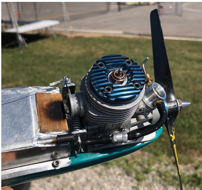
The "Flippy" end of Tim Stone's Slow Rat, GO .25 for power. Note the "scorched" plywood heat shield glued to the fuel tank to prevent erratic runs.
