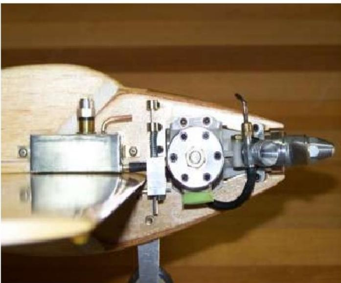
Figure 3. Installed shutoff as fitted to the airplane. Note that the position of the mounting screws in the bonded mounting plate allows assembly access. To avoid
