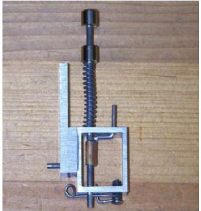
Figure 1. Rear view of the assembled F2CN shutoff in the “off” position. The frame is made from 3/4” square aluminum extrusion. Trip wire located on the bottom, and the pushrod loop located very close to the fuselage. Spacer block and mount to suit the installation held together with JB Weld.
