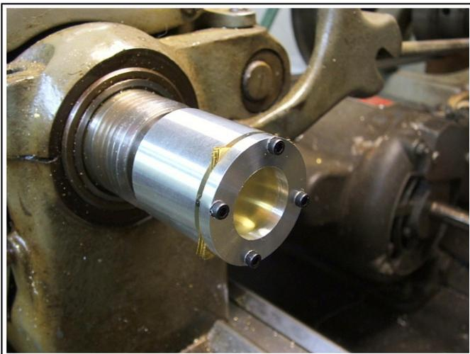
First, squares of shim material are cut to fit the ID fixture. I used a cheap paper cutter to cut .003" and .005" shim stock for these shims. Next I loaded the shim material squares in the ID fixture, placing the thicker .005" shim material on the outsides of the stack to reduce the chance of tearing the outside pieces. Tighten the four screws to compress the shim material stack so that slipping does not occur.
