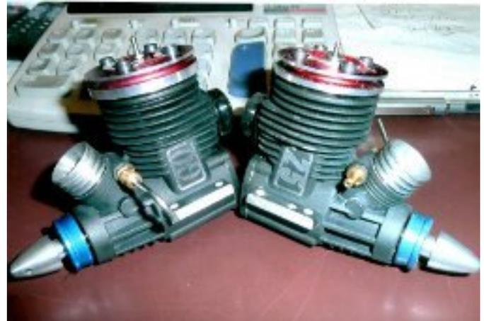
A pair of GO .25 truck motor conversions from Raul Diaz. Supertigre needle valves, Novarossi thrust washers & custom head, spinner nut & venturis.
