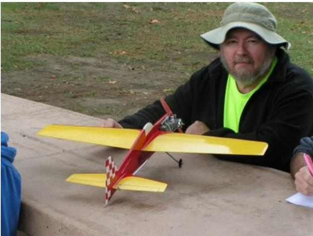
The Kusik's new Lil' Quickie SCAR Goodyear. It has an aluminum pushrod and a new style "push-to-shut-off" Dirty D shutoff. The whole works is powered by an OS .15 with a modified head. Photo: Melvin Schuette
