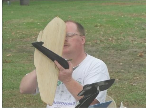
Intense concentration as Les Akre prepares his winning F2CN entry. Note the recycled F2C wing, F2C wheel, and the big chunk of lead in the tail. The Clown racer in the foreground was no slouch, either. Black paint seems to make his planes go just a bit faster. Photo: Melvin Schuette
