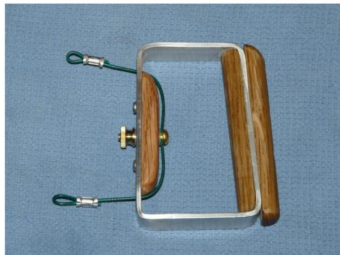
Now that you have a frame with a nice comfy grip on it, let's make the cable adjuster. First you need to know what line spacing you want. The handle shown is 3". Drill 1/8" holes through the handle frame at the desired line spacing, and drill two 1/8" holes at about a 2" spacing. Also drill a 1/8" hole in the center. Be sure to de-burr the holes where the cable passes through the handle frame.
