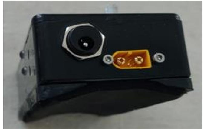
Since the back of the box is flat, not curved like the box Bill used, I added two wedge-shaped runners on the bottom, then a layer of 1/8” foam padding, to conform more to the shape of my arm. This shape, coupled with the light weight, makes attachment to my arm with only a single wrap of the elastic/Velcro work completely satisfactorily. Note, too, the DC power barrel jack for charging the battery.
