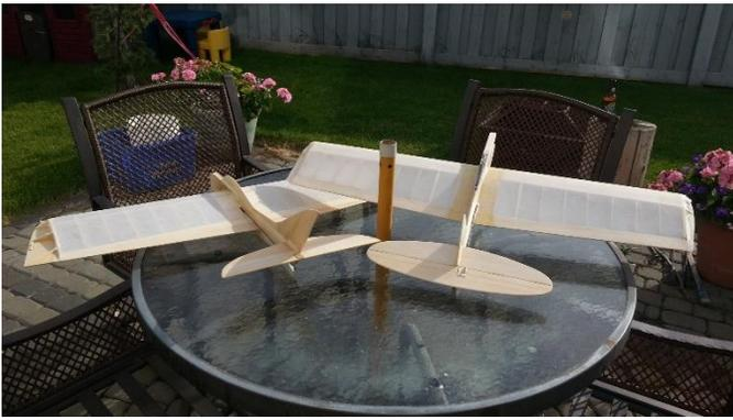
**Both Flite Streak & Ringmaster are drying outside after the Polyspan has been applied.**
