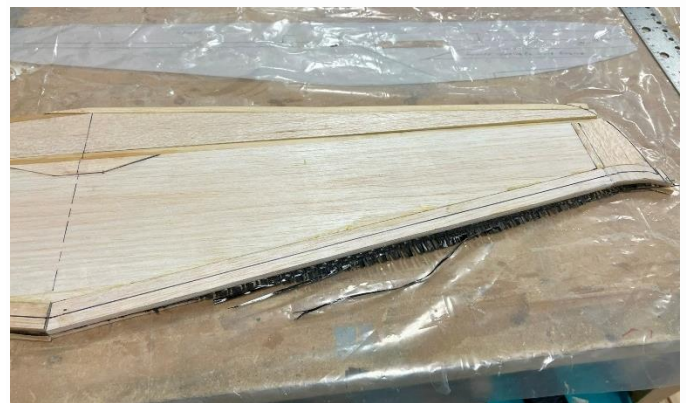
A couple more images of Gerry's Nemesis model coming along. Here's the trailing edge treatment. In Gerry's words... I've sandwiched a couple pieces of 3/16" balsa with CF in between to make up the trailing edge. First shot is the oversized chunk glued to the trailing edge.
