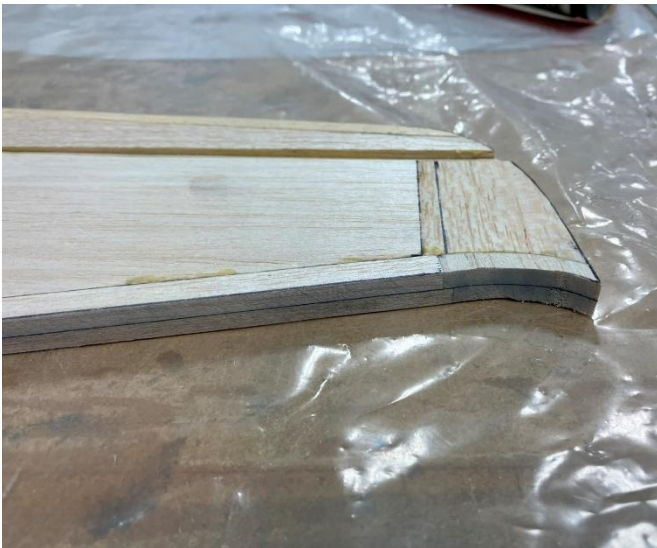
Here's the final wing profile with the 1/4" TE sandwich trimmed to shape.
