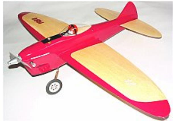
Here is a picture of Australian John Hallowell's new lightweight "Rocket" BTR. O.S. Max 25FP, 7x7 APC, 21oz.
