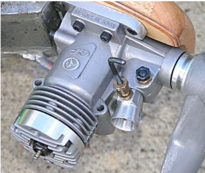
Thunder Tiger .25 with Super Tigre X-15 rear rotor venturi and G-15 needle valve assembly installed.
