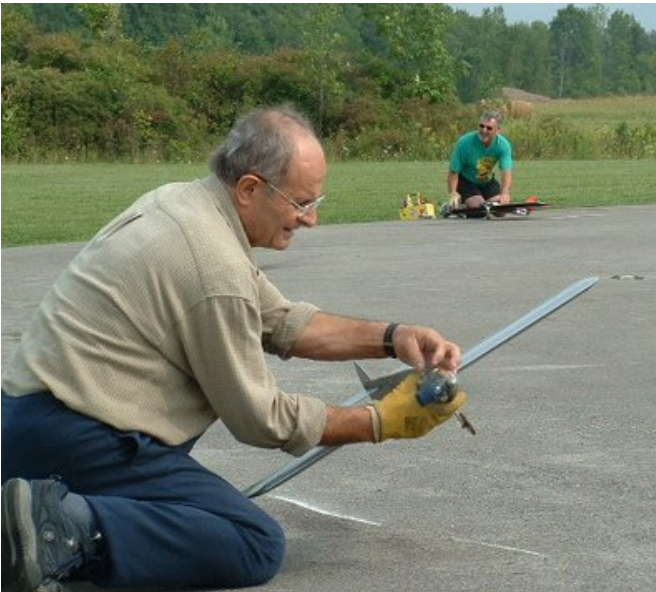
Steve Stefanovic setting the needle on his LA .25 powered Sport Racer at the Eastern Control line Championships.
