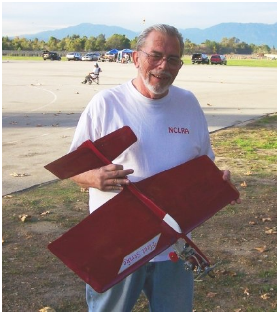
John Bruman shows off one of his new Fleet Strike Slow Rats. This original design uses a large stabilizer and elevator. Has unique adjustable/replaceable tailskid. John put up a test flight at the Toys For Tots contest and McSlow reported it grooved solid and did not appear to be tail heavy. (Photo: Hull)
