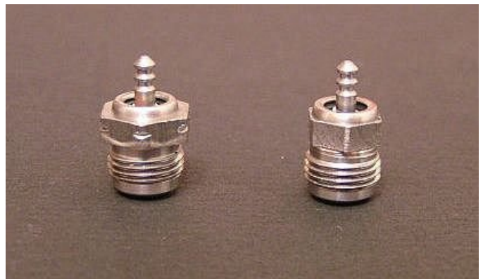
Stock Nelson plug (left), and after machining the hex to fit a Ni-starter (right).
