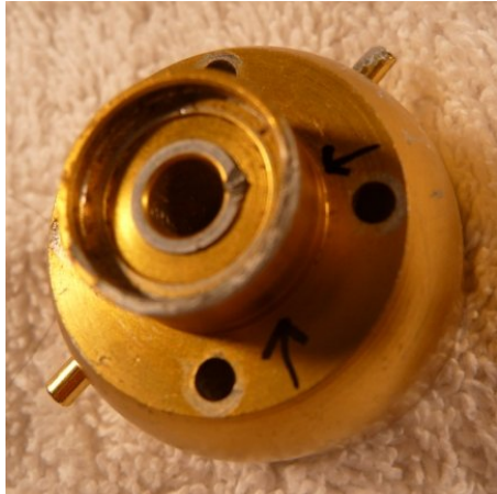
Golden Bee tank with damage to both reed sealing area and reed retainer area.
