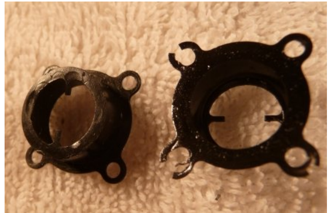
Damaged reed retainers: RT: tangs cracked, causing leaks LF: crankpin has gouged top of retainer.
