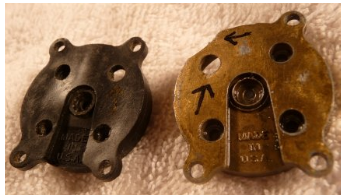
Damage to tank back hole areas & missing mounting lug
