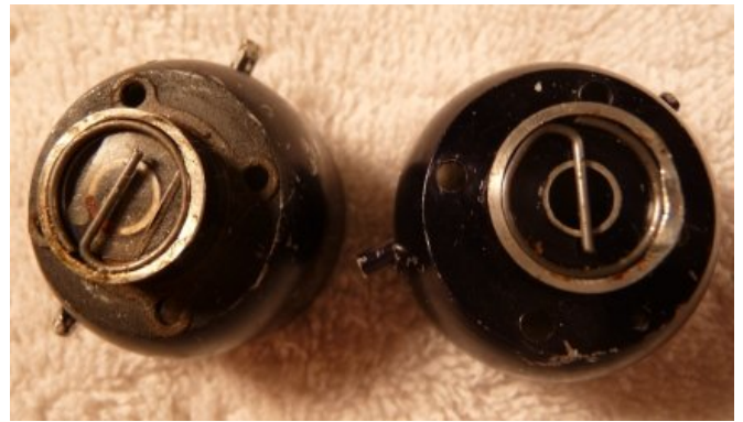
Black Widow tanks with severe wear in reed retainer (G-clip) area and wear on reed seating area.
