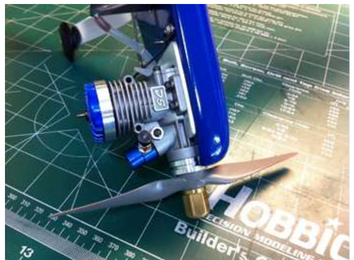
The "SC" marked .15 as sold by Hobby Partz appears to be the same as the "ASP" or "Magnum" engines.
