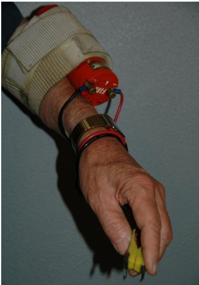
Battery strapped to arm, QuickClip readily available to attach to engine.
