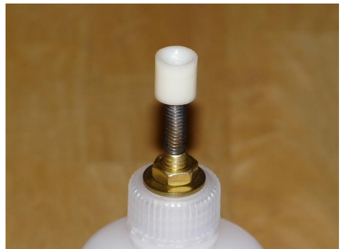
Topside View of Filler Valve.
