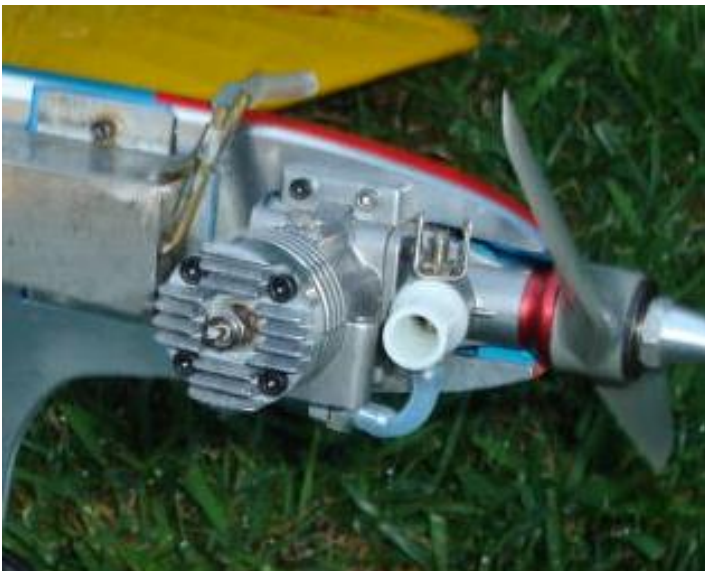
The Business end of Pete Cunha's new SSR. Note the Enya SS25EX plain bearing ABC engine for Power.
