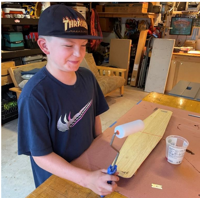
Tristan helping with the layup for wing fibreglassing.
