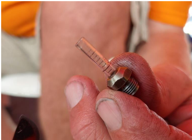
Head Chamber Volume checking tool when you just have to know precisely.
