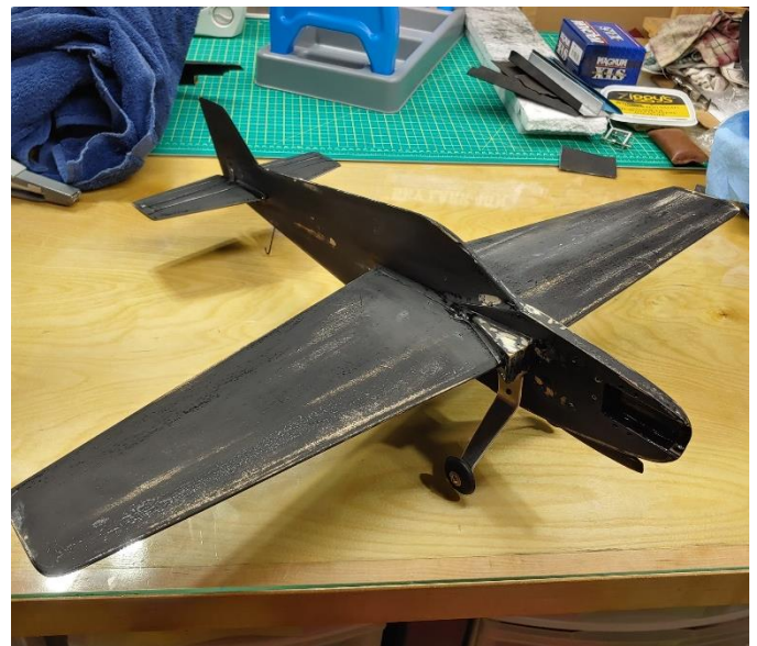
Sticky clear coat all washed off with acetone & block sanded back down with many hours & lots of 230 grit sandpaper!
