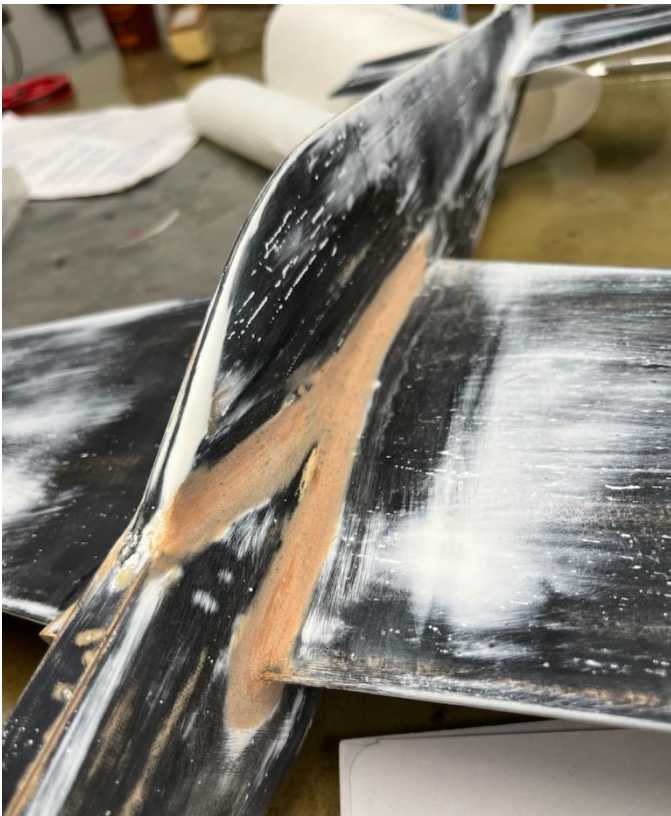
Superfil was used to do the final filleting to get everything to “flow” better.
