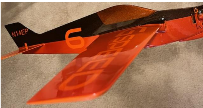
The final HOC clear is sprayed on with Candy Tangerine and Metallic added.
