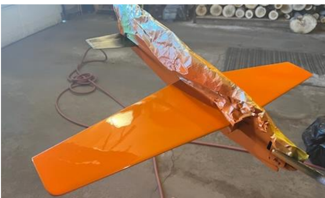
Next the hot orange is applied.
