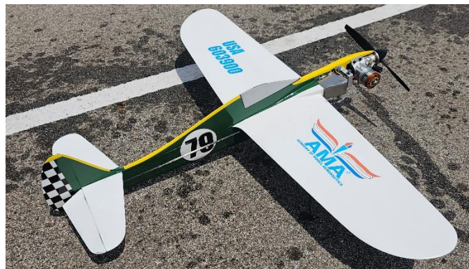
Alex Tuponov campaigned this Fora .15 Jr. powered Shoestring called "No Strings Attached" in three separate scale race events to good effect. Very Light model at 16.5oz.
