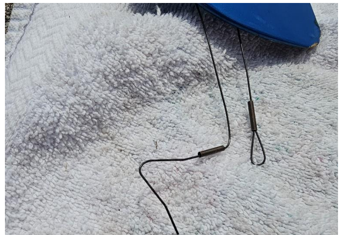
The sole crash of the TQR Nats was a model belonging to Bill Bischoff. The reason for the crash was found to be a leadout connector which pulled apart in flight. The model did however did pass a pull test just prior.
